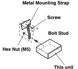
When your vehicle has the Bracket, mount the long hex bolt onto the rear panel of the CDE-9874R/CDE-9874RR/CDE-9874RB/CDE-9872R/CDE-9872RM/CDE-9872RE and put the Rubber Cap on the hex bolt. If your vehicle does not have the Mounting Support, reinforce the head unit with the metal mounting strap (not supplied). Connect all the leads of the CDE-9874R/CDE-9874RR/CDE-9874RB/CDE-9872R/CDE-9872RM/CDE-9872RE according to details described in the CONNECTIONS section.
